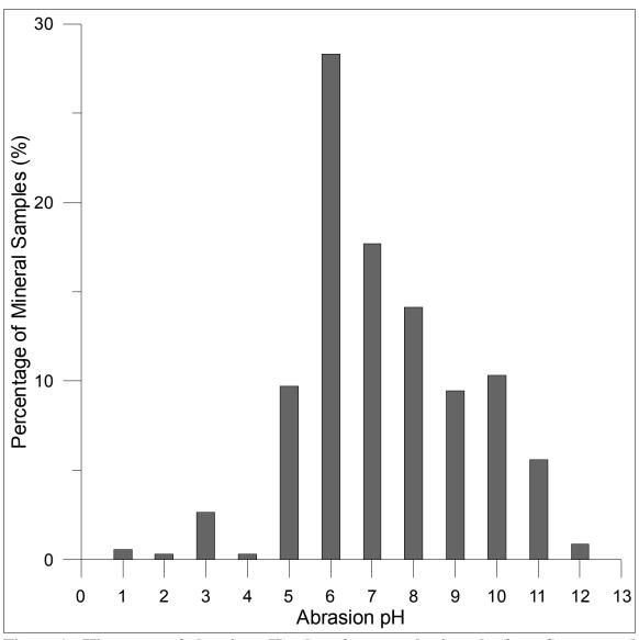
Figure 1. Histogram of abrasion pH values for several minerals (from Stevens and Carron, 1948).
