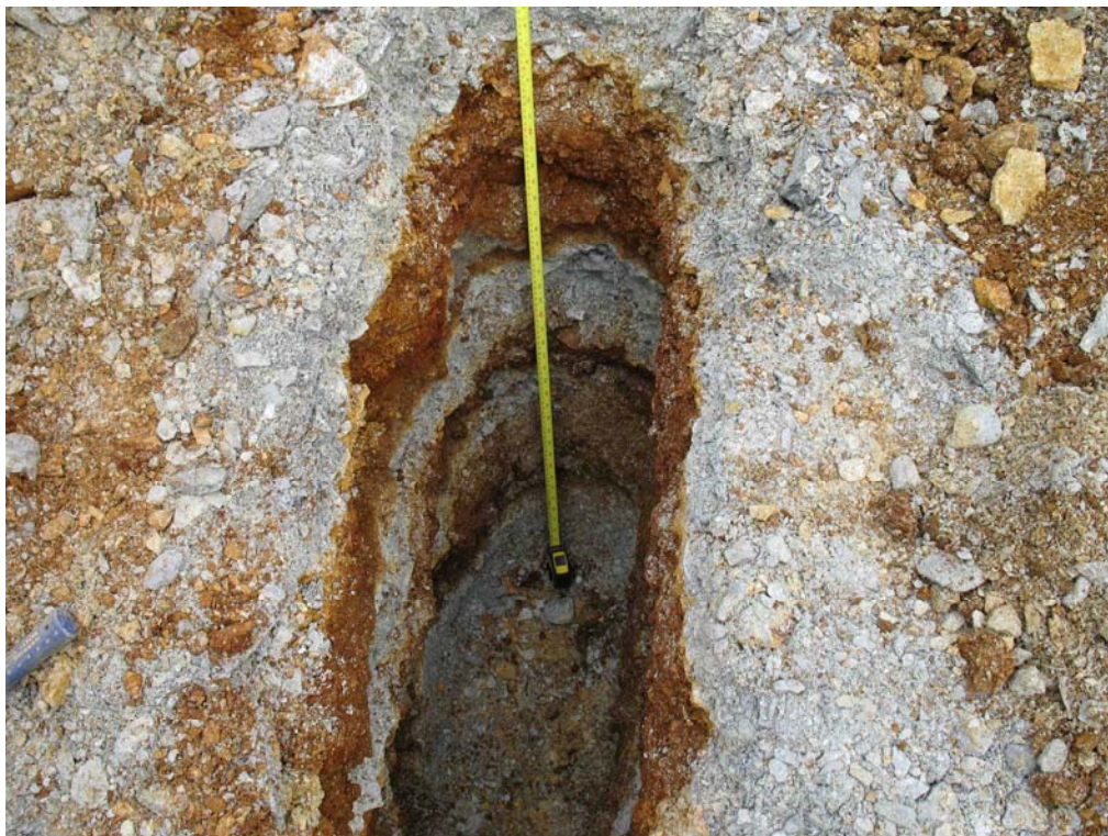
Five-Year-Uncovered Crib – Closer View of Trench (Note the distinct light-grey and orange-brown layers).
