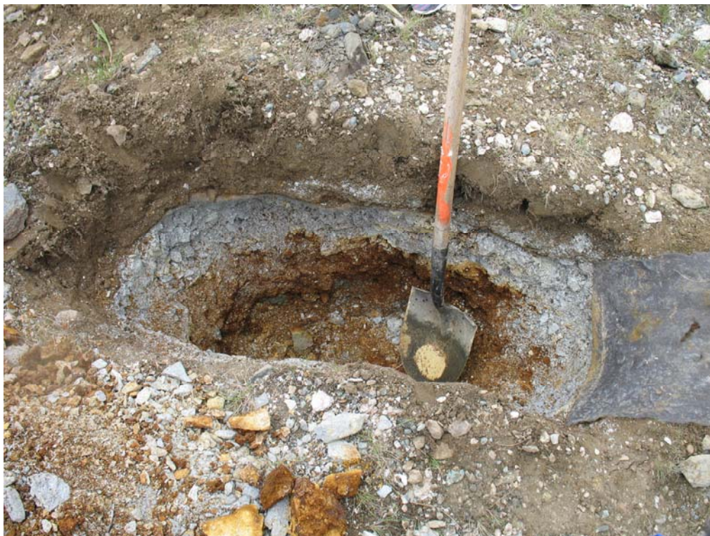
Five-Year-Covered Crib - View of Initial Trench (Note the distinct light-grey and orange-brown layers).
