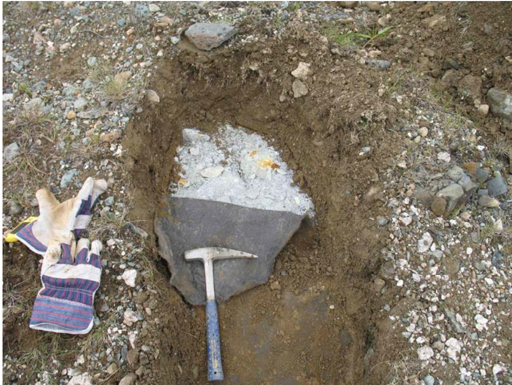
Five-Year-Covered Crib – Initial Trench Excavation, Showing Filter Cloth Between the Uppermost Till and Underlying Light-Grey Mine Rock.
