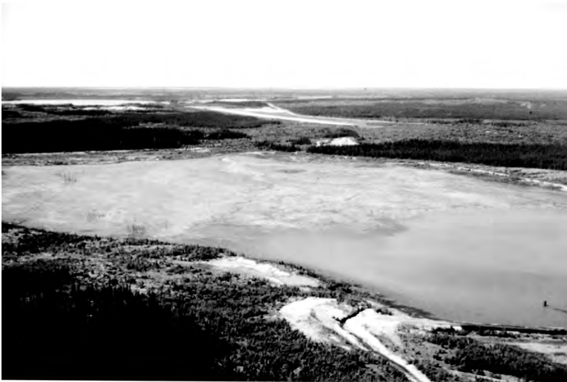
Oblique Air Photograph of a Tailings Impoundment.
